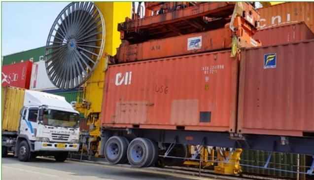
The application LaseTLP - Truck Lifting Prevention ensures a lifting prevention of truck-trailers during the hoist process caused by locked twistlocks.
